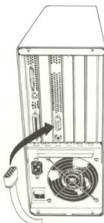
Figure 10-1. Connecting an Industry-standard Monitor
