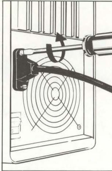
Figure 10-2. Connecting the Power Cord
